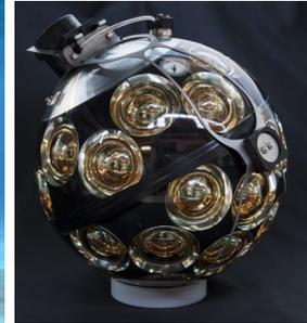
**Figure 1.2:** An optical detector (DOM) *source:*
